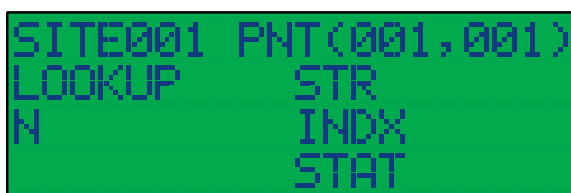
Fig.7.2.2 Screen When Recorded Data Does Not exist
