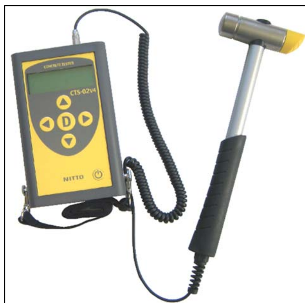
Fig.6.2-1 Instrument Body and Hammer Unit
