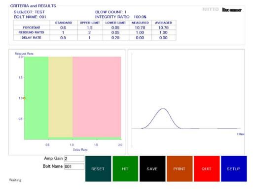
Figure 4-2 After measurement
